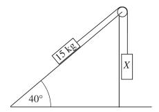
(a) The 15 kg mass accelerates down the slope at 0.50  $\rm m\,s^{-2}.$
