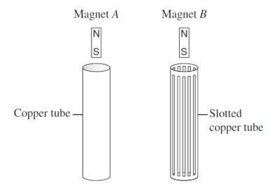
The magnets are dropped simultaneously. Each magnet falls straight through its tube without touching the tube walls.
